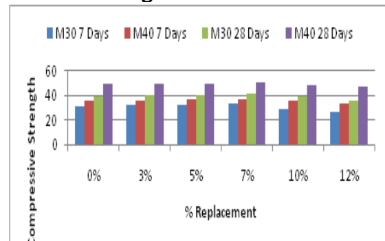
Graph 3: Comparison of compressive strength of different mixes of Brine Sludge Concrete
