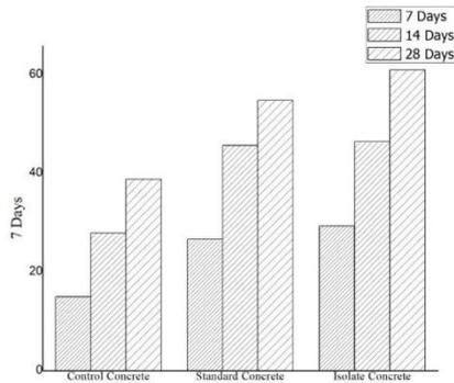
**Figure 4 Compressive strength of control, isolate and standard concrete at 7, 14, 28 days respectively**
