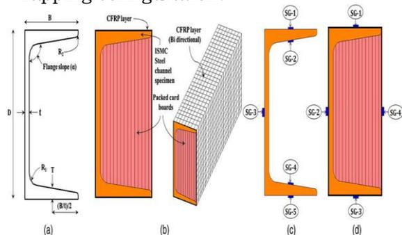
**Fig.3. Test specimen: (a) cross-sectional dimensions of ISMC 75 specimen; (b) view of the ISMC specimen packed with cardboard and CFRP wrapping; (c) location of strain gauges at mid span for wrapping configurations B, S<sub>1U</sub>, and S<sub>1B</sub>; (d) location of strain gauges at mid span for wrapping configurations C<sub>1U</sub>, C<sub>1B</sub>, C<sub>1U\_1B</sub>, and C<sub>2U\_1B</sub> [10].**
