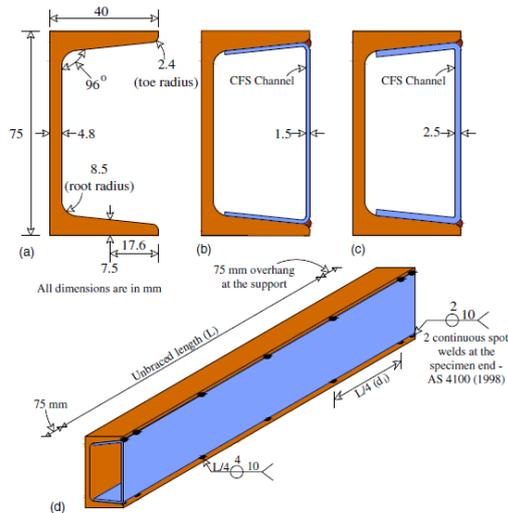
**Fig.2. Test specimens: (a) control specimen; (b) retrofitted specimen with 1.5-mm-thick CFS channel; (c) retrofitted specimen with 2.5-mm-thick CFS channel; and (d) details of interconnection (spot welding) [11].**
