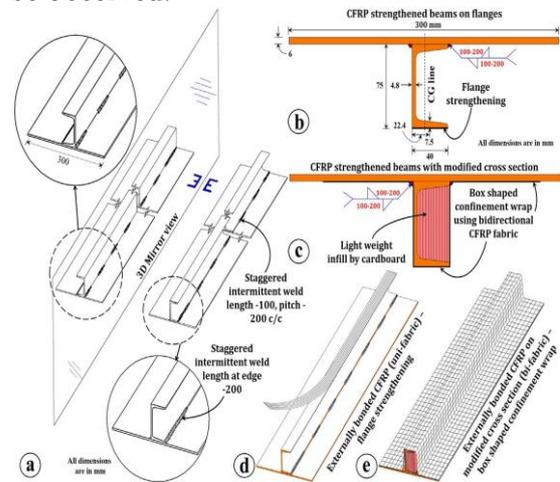
**Fig.10. Built-up test specimen fabrication: (a) 3D normal and mirror view welding details; (b) Cross sectional view of the flange strengthening specimen; (c) Cross sectional view of the modified cross section strengthening specimen; (d) CFRP bonding method on flange strengthening specimens; (e) CFRP bonding method- box shaped confinement wrap [9].**
