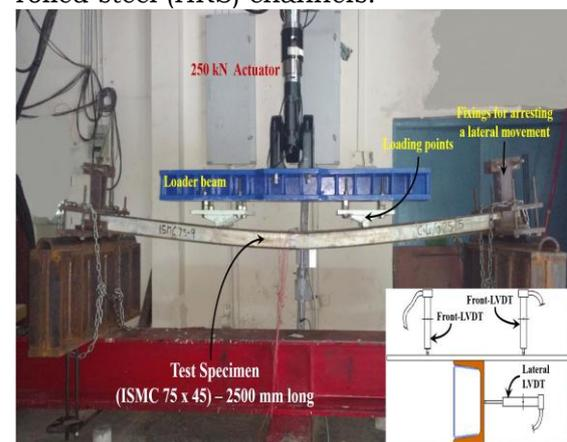
**Fig.1. Four-point bending test arrangement (LVDT = linear variable displacement transducer) [11].**
