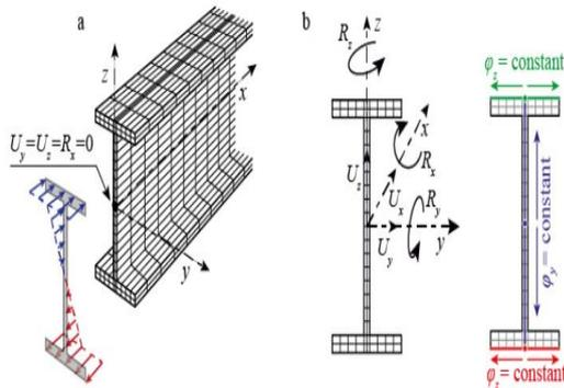
**Fig. 5. Ansys solid model (a) loading; (b) kinematic coupling constraints.**
