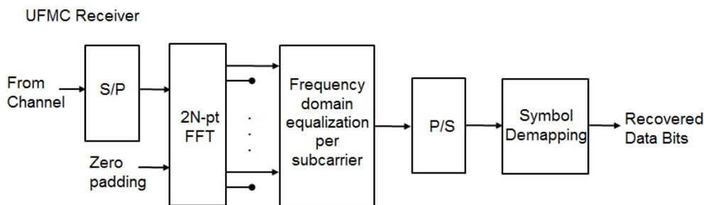
**Fig.3: Block Diagram of UFMC receiver**
