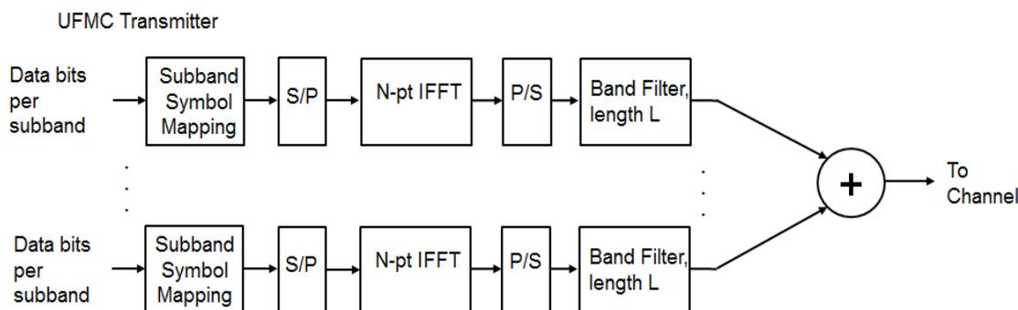
**Fig.2: Block Diagram of UFMC transmitter**
