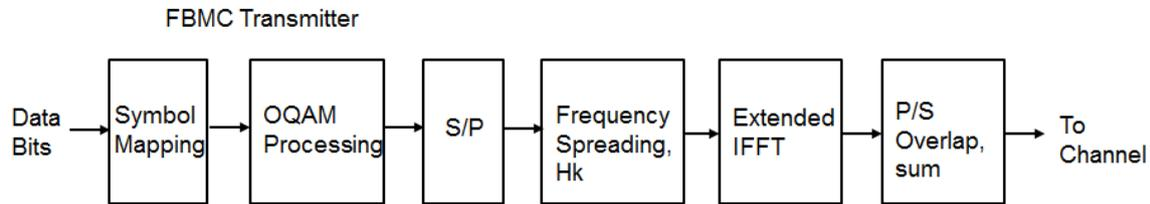
**Fig.4: Block Diagram of FBMC Transmitter**
