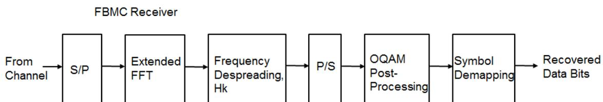
**Fig.5: Block Diagram of FBMC Receiver**
