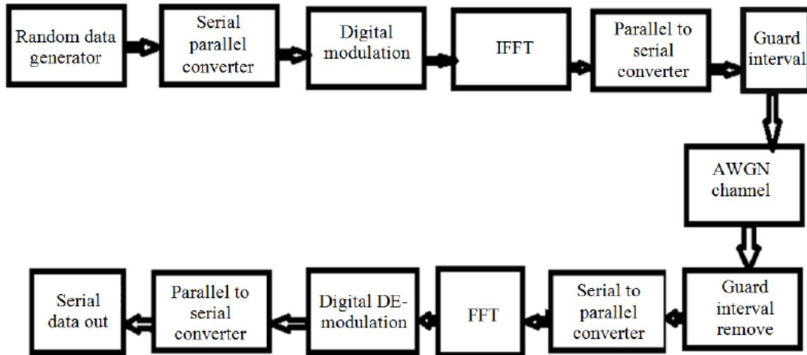
**Fig.1: Block Diagram of OFDM**
